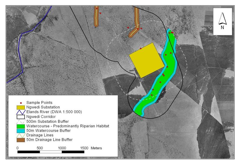
Figure 2: Demarcated watercourses and their associated buffers around the Ngwedi Substation, the south-eastern portion of the Ngwedi Corridor (associated with a separate transmission line project), and a 500 m buffer around the substation.
